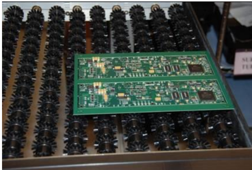
Figure 35: Uncontrolled Brushes Generate > 500 V on PCBs
